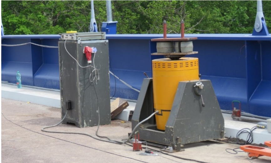
Figure 5. The view on the electrodynamic shaker TIRAVIB 5140 situated on the bridge deck.
